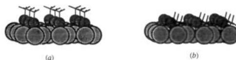
Figure 13. A nine-molecule section of a fully-covered SCH 3 monolayer on Au(111) minimized with a modified MM2 force field including the (a) sp and (b) sp 3 chemisorption parameters. We have used one molecule per unit cell with periodic boundary conditions and a nonbond cutoff of 9 Å. The gold atoms are shown in light gray having their full van der Waals radii. The sulfur atoms are shown in dark gray and are not drawn to scale.
