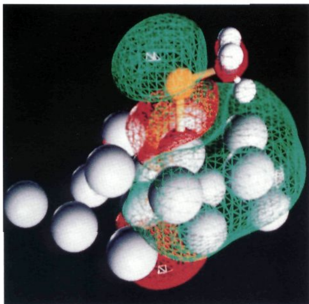
Figure 5. The \sigma -bonding orbital of \text{SCH}_3 to the \text{Ag}(111) surface in the on-top position.
